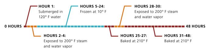
48 hour test cycle completed 6 times. Now that is durable!
